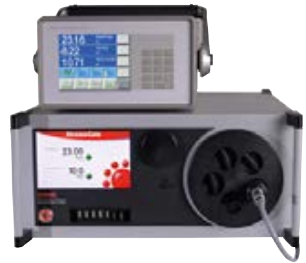
HygroGen2 with external MBW473 dew point reference
