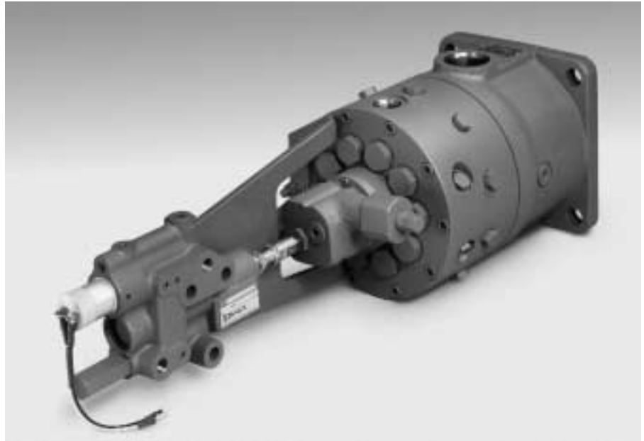
A Remote Proportional Actuator can control a Dynex mechanical variable delivery checkball pump. Output flow is controlled by stroking the spring-biased volume control stem at the back of the pump.
