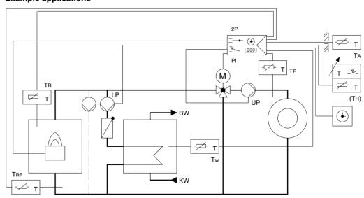
Weather-dependent supply-temperature control with precontrolling of the boiler temperature and the domestic-hot-water control
