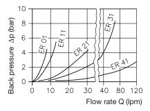
$\Delta$ p-Q curves (guideline) Oil viscosity during tests approx. 60 mm<sup>2</sup>/s
