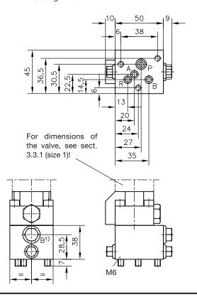
Holes in the manifold and sealing of the ports by O-rings <sup>2</sup>)
