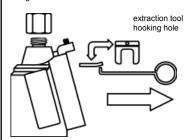
Extract the clip putting the extraction tool (KM/3062) in the hole of the security clip then pull hard to extract Extract the solenoid housing and the solenoid from the solenoid valves pulling up. Solenoid housing and solenoid will remain connected to the power supply cable.
