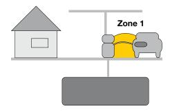
Any device certified for zone 1 must be group IIA, IIB or IIC and at least category "ib".
