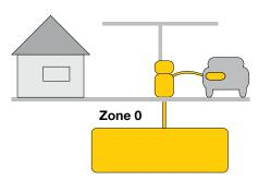
Intrinsically safe devices designed for use in zone 0 must meet category "ia" safety standards and must have no live contacts. Galvanic isolation between intrinsically safe and non-safe devices is to be preferred. If grounding of the intrinsically safe circuit is required for functionality, this must be done outside zone 0, but as close as possible to zone 0. The devices must as well be approved for gas groups IIA, IIB and IIC.
