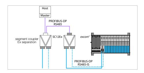
The GDP-IS gateway serves to connect the excom® system to PROFIBUS-DP networks. Connection to the PROFIBUS-DP is established via fiber optics or copper cables. The use of fiber optics for data transfer requires the connection of a coupler pair between wired and optical PROFIBUS and also for level adjustment to the IS layer. When using copper cables it is required to install a segment coupler (RS485-IS coupler) to ensure explosion protection.
