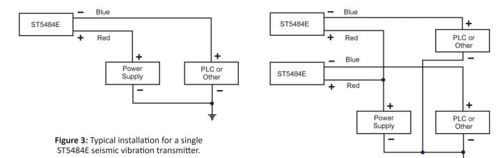
**Figure 4:** Typical installation for multiple ST5484E seismic vibration transmitters.
