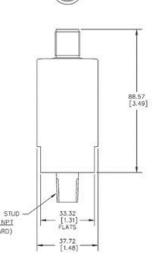
**Figure 1:** Outline dimensions of the ST5484E (all versions except MIL-Style Connector). Dimensions in mm [inches]. Optional\* 8200-001 conduit elbow shown installed.
