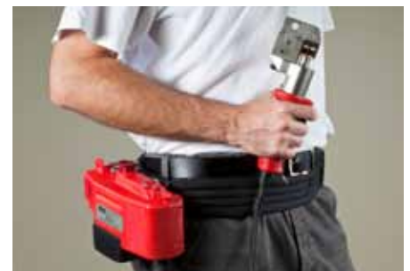
The battery and pump unit can be worn on a tool belt (p/n 2063863-1) ...
