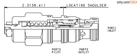
Counterbalance valves with pilot assist are meant to control an overrunning load. The check valve allows free flow from the directional valve (port 2) to the load (port 1) while a direct-acting, pilot-assisted relief valve controls flow from port 1 to port 2. Pilot assist at port 3 lowers the effective setting of the relief valve at a rate determined by the pilot ratio.
