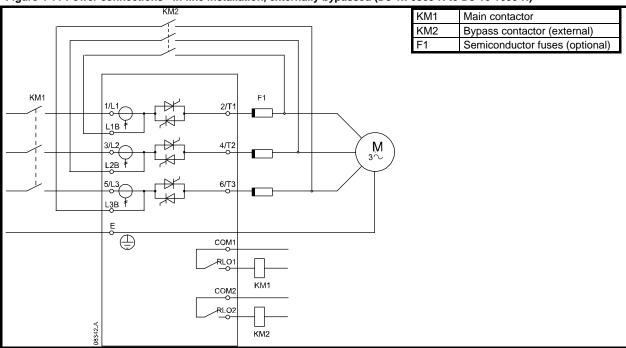
NOTE The bypass terminals on D3-1x-0255-N are T1B, T2B, T3B. The bypass terminals on D3-1x-0360-N to D3-16-1600-N are L1B, L2B, L3B.
