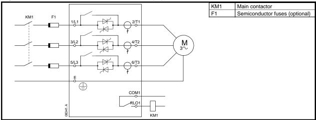
NOTE Main contactor is the default setting for Pr 4A Relay A Action (COM1, RLO1).
