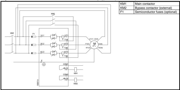
Figure 4-15 Power connections - inside delta installation, externally bypassed (D3-1x-0360-N to D3-16-1600-N)
