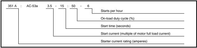
**Starter current rating**: The full load current rating of the soft starter given the parameters detailed in the remaining sections of the utilisation code.
