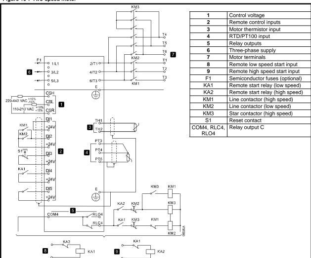
NOTE Contactors KM2 and KM3 must be mechanically interlocked.
