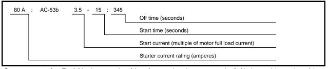
Starter current rating: The full load current rating of the soft starter given the parameters detailed in the remaining sections of the utilisation code.
